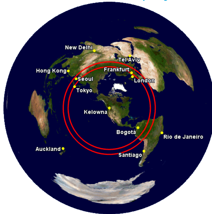
Figure 36: Runway 16-34 Maximum Geographic Ranges for B767-300ER Take-offs from OLS Protected Runway Lengths
